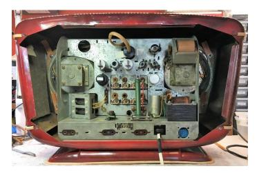
All the resistors except one were original carbon film radial 'dogbone' construction with Russian markings and all tested within tolerance. The single replacement was a 470k carbon composite
