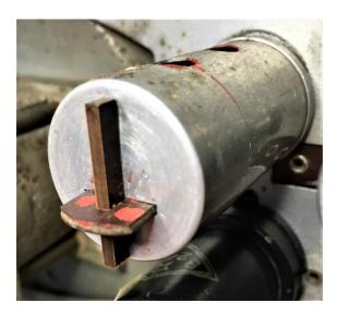
The threaded slugs were then held in a vise with rubber jaws, tiny drops of JB KwikWeld applied to the broken tops, and new slots cut with a small hacksaw.
