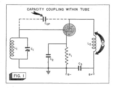
through the receiver over feedback paths. This reversal of the normal direction of signal movement can occur only when there is an undesired coupling between circuits in the same stage or in different stages. This coupling may be inductive coupling, or may be stray capacity between circuit wires or within tubes.
