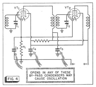
plate currents can get into the power supply leads and be coupled to other circuits in the right phase to cause oscillation. Although  $C_5$  is in parallel with the output filter condenser, the filter condenser cannot assume the function of  $C_5$  because electrolytics have higher power factors than do paper condensers, and also they are inductively wound; both conditions make them poor r.f. by-passes.
