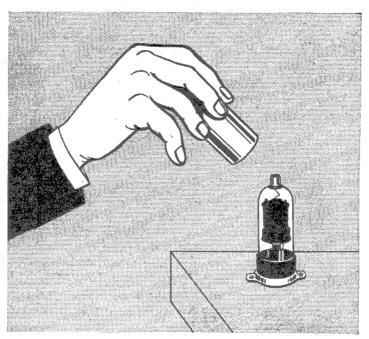
A missing shield is often the reason why a set goes into oscillation. Whenever you remove a shield from a tube, be sure to replace it before considering the repair finished. Do not depend on the operation of the set to tell you whether a shield is missing; it is entirely possible for a set to work properly for a while with a missing shield, only to go into oscillation later on because, say, the characteristic of some tube changes.
