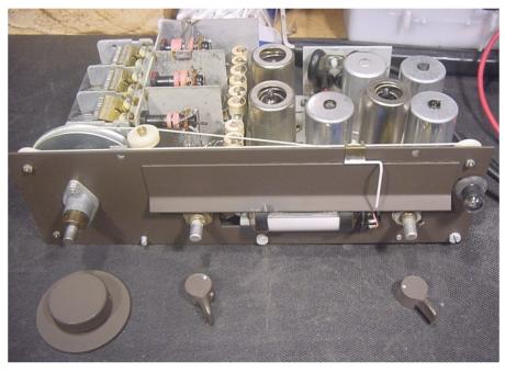
taking parts of the gold paint with it, the result being rather unattractive (photo, top of Page 6). The tuner chassis is enclosed in a pressed metal enclosure that matches other QUAD HiFi components of the period (photo on page 6) – this was really designed to be installed in a larger enclosure, as was the vogue in the 50's and 60's for this type of equipment.
