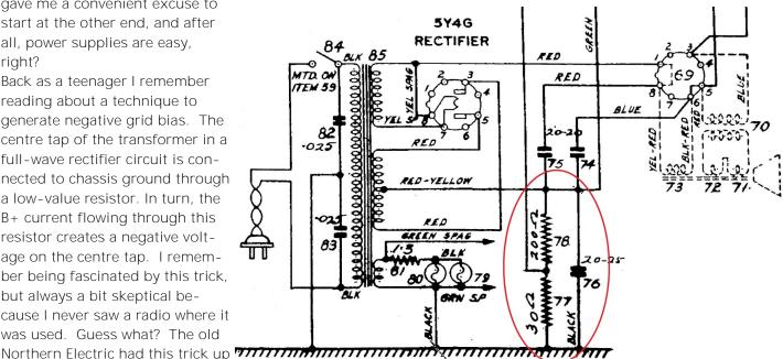
The power supply schematic is shown right. You can see that the centre tap on the transformer secondary is connected to ground through a 200 ohm and a 30 ohm resistor in series. Current through these resistors results in the
