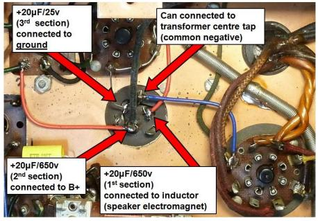
cuit, the positive lead of the capacitor is connected to the chassis ground, while the negative lead (the can) remains connected to B- at the transformer tap. The wiring is shown in the photo on the next page. A neat trick. Easy to get backwards when installing a new filter can.
